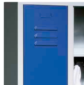
Sturdy steel construction: Doors hinged on the right, mounted on fulcrum pins with center reinforcement for high stability, vent slots, and stamped-in label holder.
